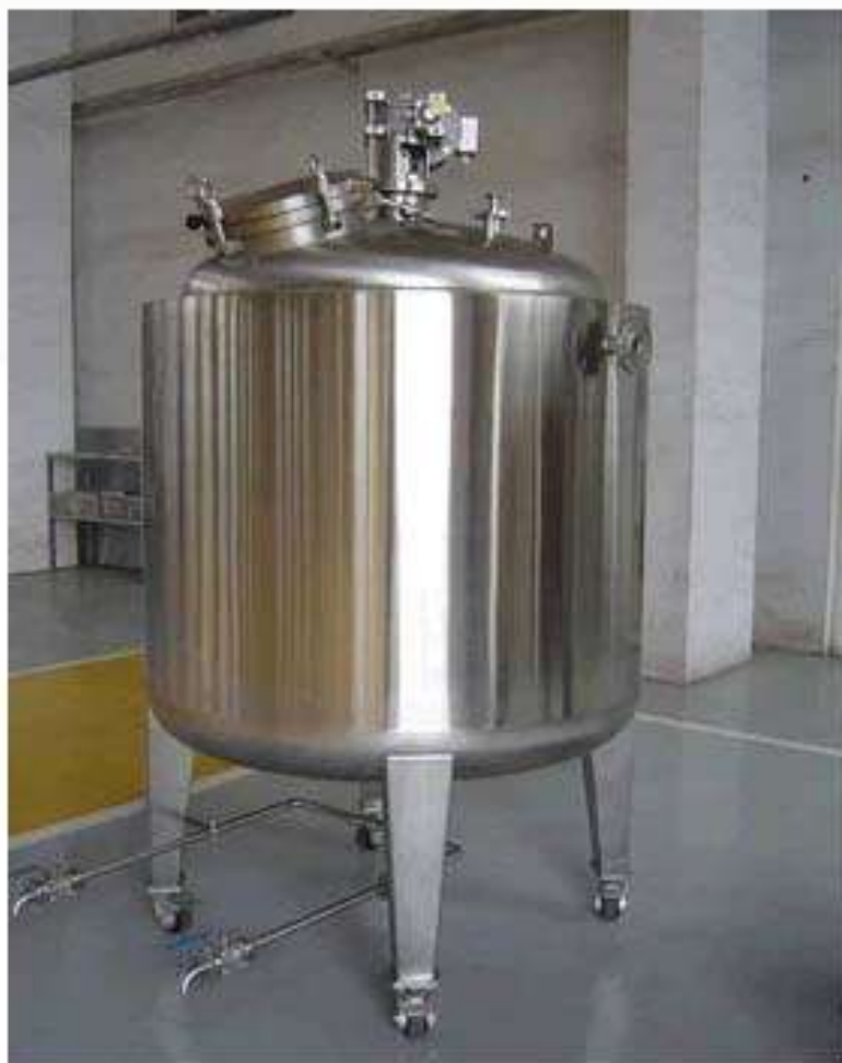
Steam jacketed Vessel Herbal Extraction vessel
